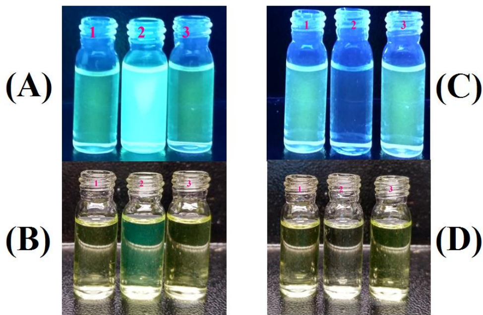
Figure 4.20 Visual colour changes in reversibility experiments. For (A) and (B), 1= Only HL4.1 (10µM), 2= HL4.1 (10µM) + Zn 2+ (20µM), 3= HL4.1 (10µM) + Zn 2+ (20µM) + EDTA 2- (20µM) under UV and normal light, respectively. For (C) and (D), 1= Only HL4.1 (10µM), 2= HL4.1 (10µM) + Cu 2+ (20µM), 3= HL4.1 (10µM) + Cu 2+ (20µM) + EDTA 2- (20µM) under UV and normal light, respectively.
