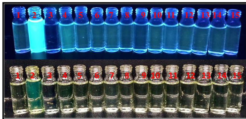
Fig. 9. Visual color changes of chemo sensor ( HL ) ( 10\ \mu\text{M} ) under presence of different metal ions ( 2.0 equivalent) in HEPES buffer ( \text{pH } 7.4 ). The images in below row and above row were taken under visible light and UV light respectively. Where 1 = only HL , 2, 3, 4, 5, 6, 7, 8, 9, 10, 11, 12, 13, 14 and 15 = HL + \text{Zn}^{2+} , \text{Cu}^{2+} , \text{Cd}^{2+} , \text{Pb}^{2+} , \text{Hg}^{2+} , \text{Mn}^{2+} , \text{Fe}^{3+} , \text{Co}^{2+} , \text{Ni}^{2+} , \text{K}^+ , \text{Na}^+ , \text{Mg}^{2+} , \text{Ca}^{2+} and \text{Al}^{3+} respectively.
