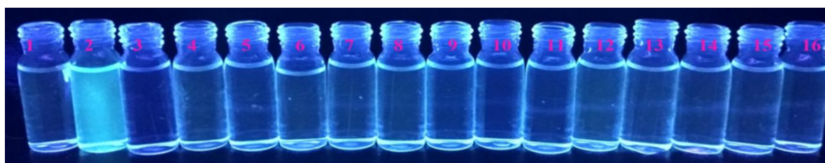
Figure 5.17 Color changes of chemosensor H 2 DTC5.1 (10 \mu M) in the presence of different metal ions (4 equiv.) in HEPES buffer (10 mM, pH 7.4). The images were taken under UV light. Where, 1= only H 2 DTC5.1 , 2-16 = H 2 DTC5.1 + Zn 2+ , Cu 2+ , Cd 2+ , Pb 2+ , Hg 2+ , Mn 2+ , Fe 3+ , Co 2+ , Ni 2+ , Cr 3+ , K + , Na + , Mg 2+ , Ca 2+ and Al 3+ , respectively.
