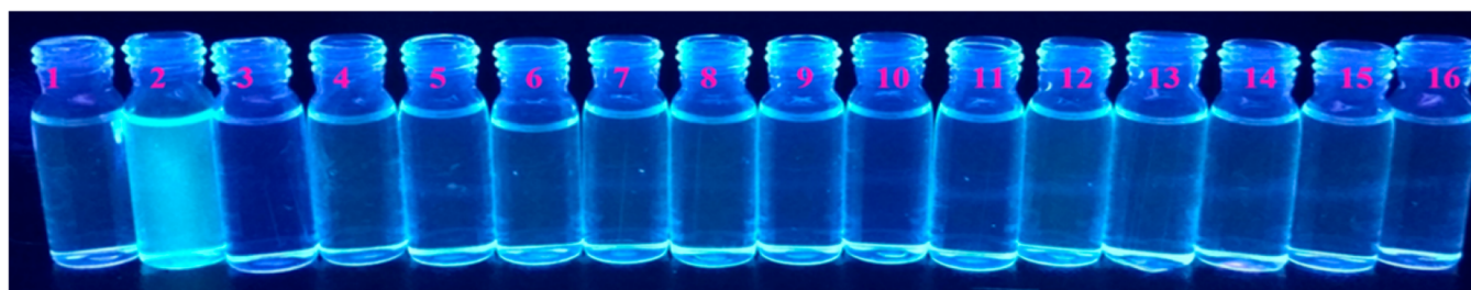
Figure 4. Color changes of the chemosensor H 2 DTC (10 \mu M) in the presence of different metal ions (4 equiv) in HEPES buffer (10 mM, pH 7.4). The images were taken under UV light. Legend: 1, only H 2 DTC; 2–16, H 2 DTC + Zn 2+ , Cu 2+ , Cd 2+ , Pb 2+ , Hg 2+ , Mn 2+ , Fe 3+ , Co 2+ , Ni 2+ , Cr 3+ , K + , Na + , Mg 2+ , Ca 2+ , and Al 3+ , respectively.
