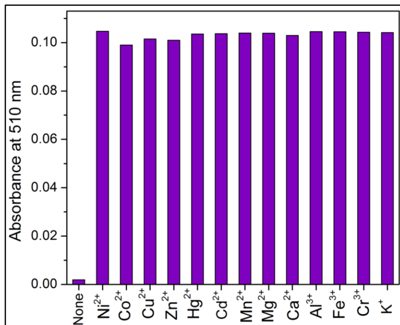
Fig. 5.4: Absorbance intensity of chemosensor (H 2 L) (10 μM) upon addition of 10 μM Ni 2+ along with various metal ions i.e, Co 2+ , Cu 2+ , Zn 2+ , Hg 2+ , Cd 2+ , Mn 2+ , Mg 2+ , Ca 2+ , Al 3+ , Fe 3+ , Cr 3+ , K + (20 μM)
