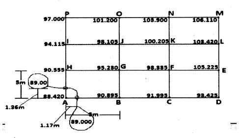
Q5. Reproduced below is the page in a level book. Fill in the missing data. Apply usual checks. [6]
