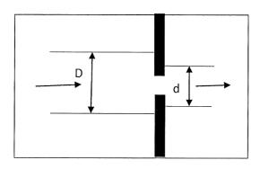
2(a) A vertical plate has a sharp-edged orifice at its centre. A water jet of speed 5 m/s strikes the plate concentrically. Obtain an expression for the external force needed to hold the plate in place, if the jet leaving the orifice also has a speed 5 m/s.
