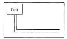
considered to be smooth. The pipe contains one gate valve; other minor losses may be neglected. The pipe diameter is 5 cm. Determine the maximum flow rate through the pipe.
