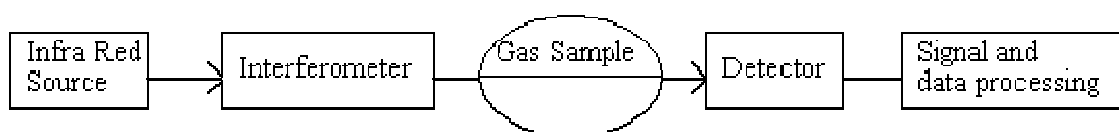
Fig. 1.3: Basic components of FTIR
