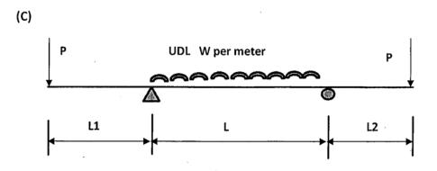
7. For the given beam and the loading as drawn in the picture below, find the values of Bending Moment and Shear Force at the locations A, B, C, D, E, and F on the beam. (16)
