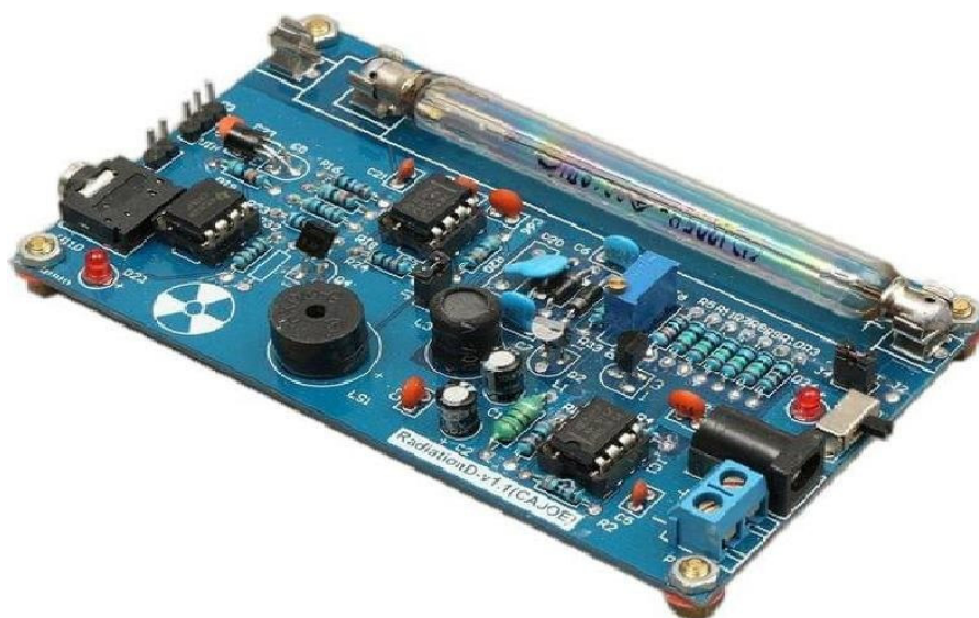
Fig. 4.7: Assembled Geiger Counter
