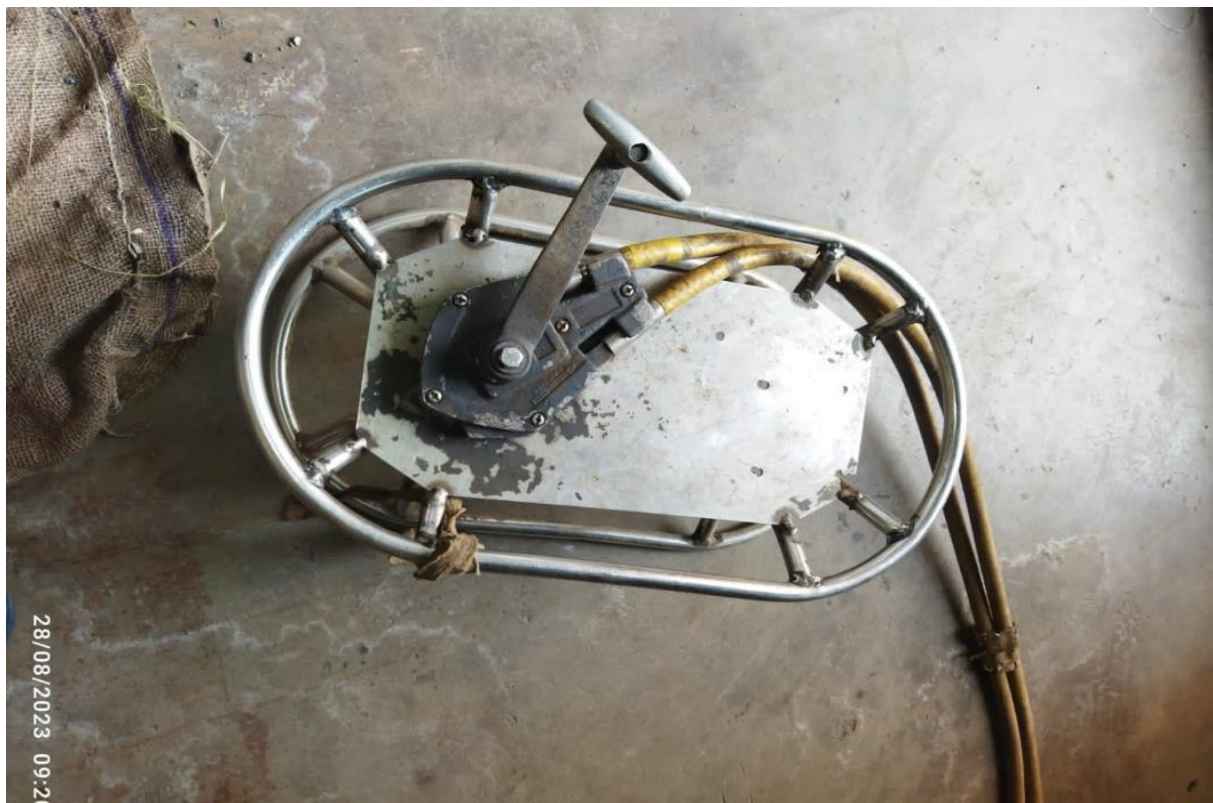
Fig. 5.3 (ii): Manual Cranking Unit of ROLI-3 IGRED
