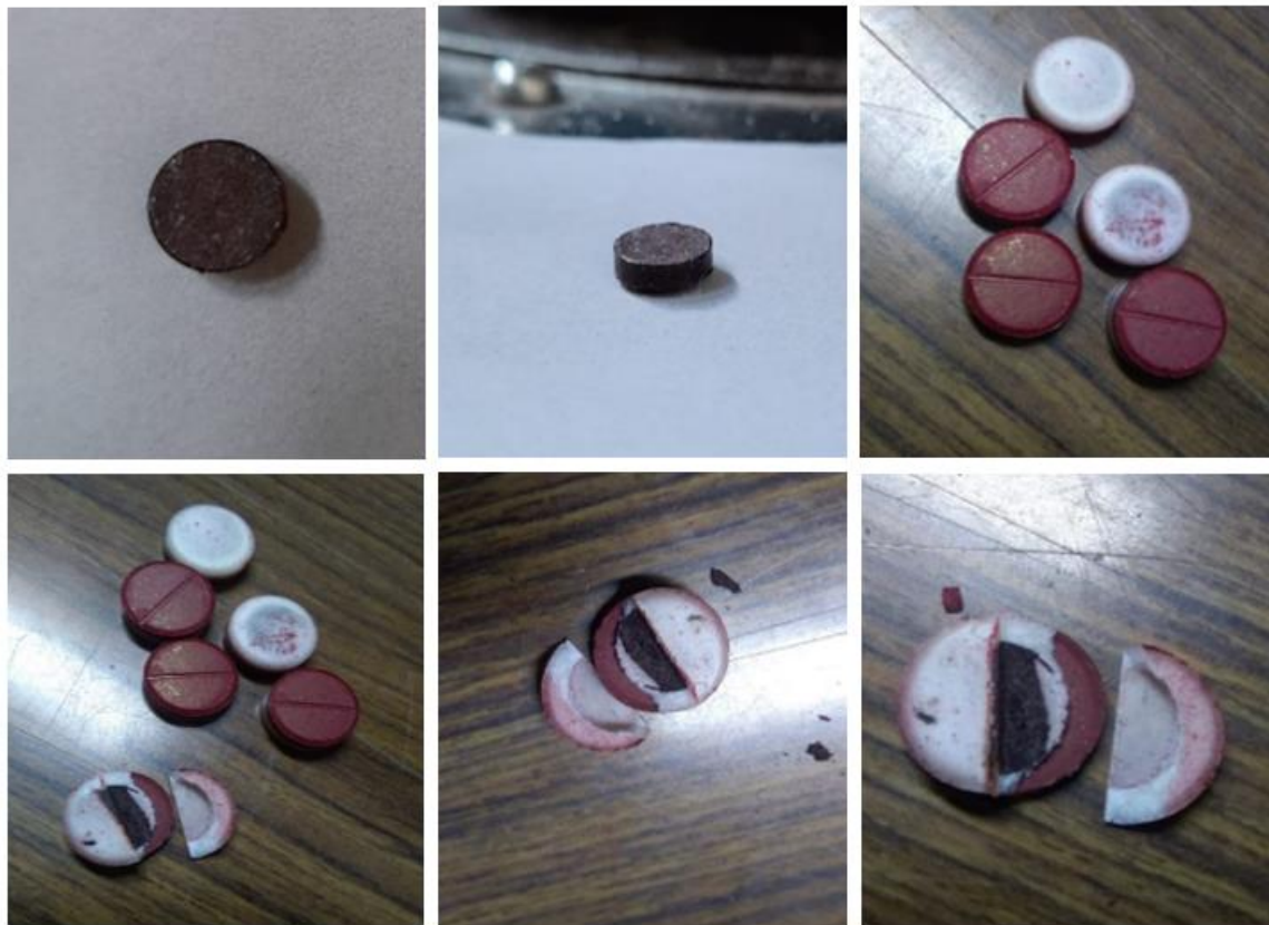
Figure 5.33. Prepared core in cup tablets
