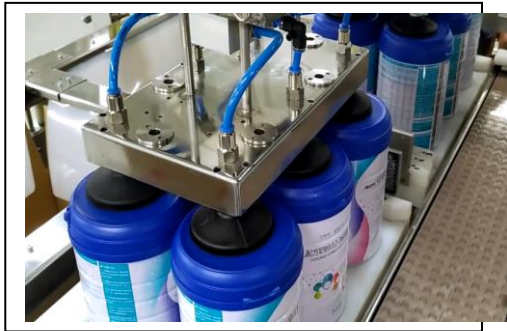
Figure 9-2: Pick & Place Machine ordered by ITC
