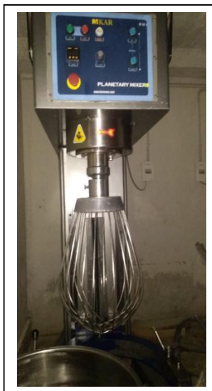
Figure 9-17: Cake Mixing Machine
