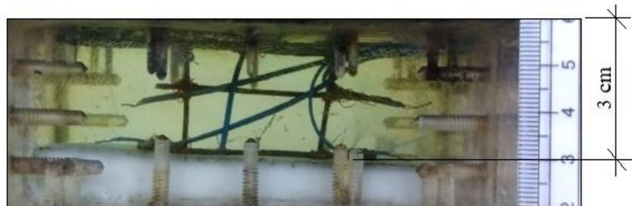
(c) Picture representing molten PCM at time t = 7:30 hours during heating
