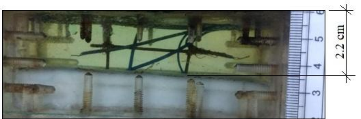
(b) Picture representing molten PCM at time t = 3:50 hours during heating
