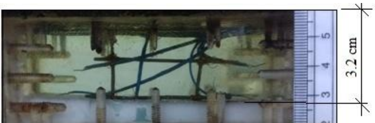
(b) Picture representing molten PCM at time t = 12 hours during heating
