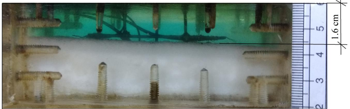
(b) Melt fraction of the PCM, captured on experiment at t=5 hours
