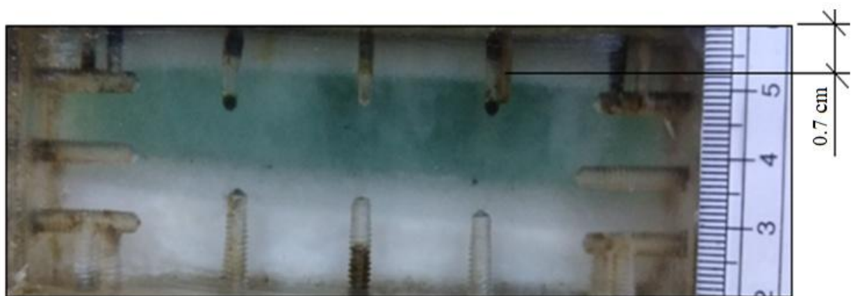
(b) Picture representing molten PCM at time t = 15:40 hours during cooling
