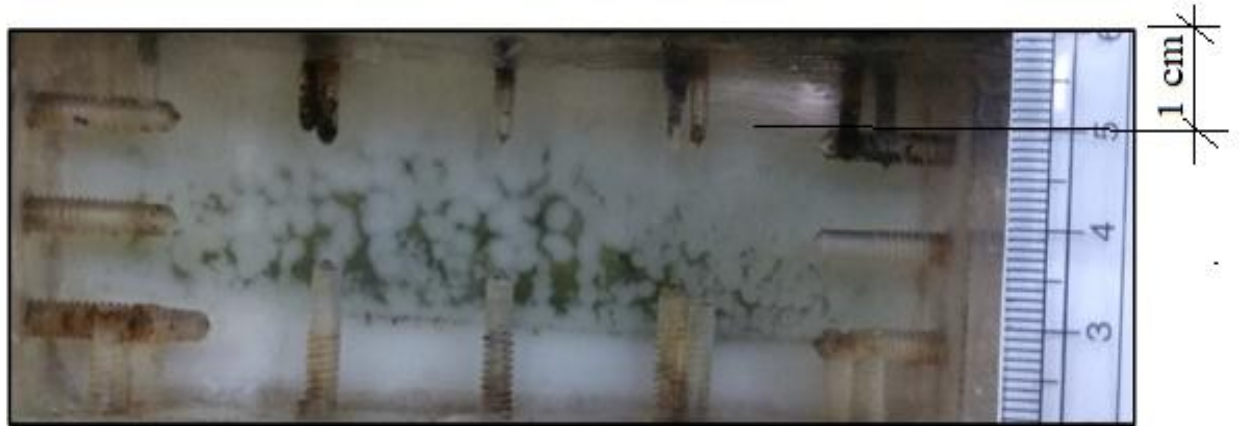
(a) Picture representing molten PCM at time t = 16:30 hours during cooling
