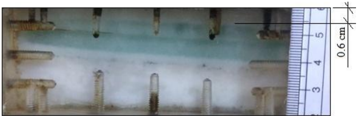
(b) Picture representing molten PCM at time t = 13:45 hours during cooling
