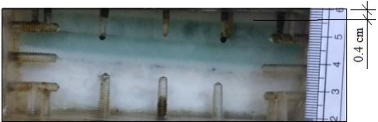
(a) Picture representing molten PCM at time t = 13:30 hours during cooling
