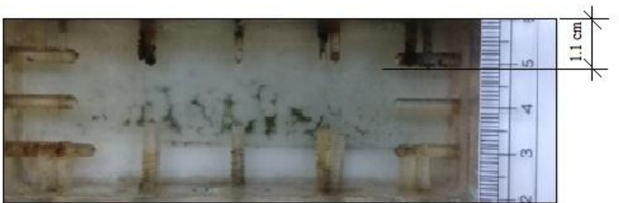
(b) Picture representing molten PCM at time t = 16:50 hours during cooling
