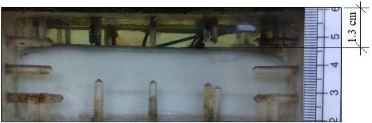
(a) Picture representing molten PCM at time t = 1:20 hours during heating
