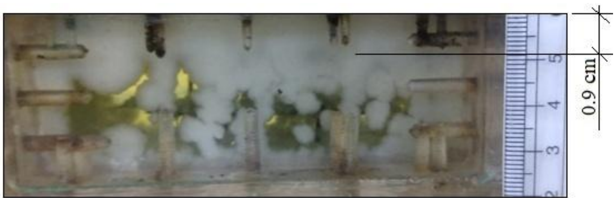
(b) Picture representing molten PCM at time t = 15:10 hours during cooling
