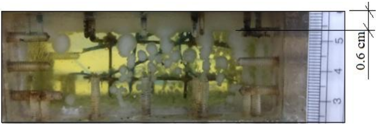
(a) Picture representing molten PCM at time t = 14:40 hours during cooling
