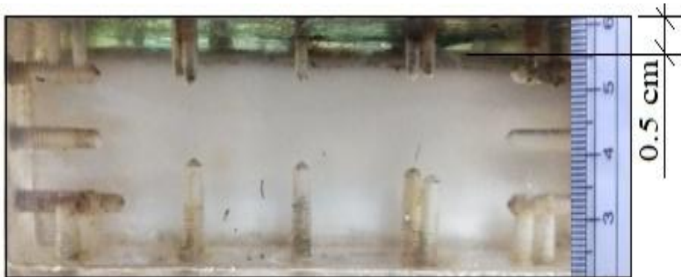
(b) Melt fraction of the PCM, captured on experiment at t=0:30 hours
