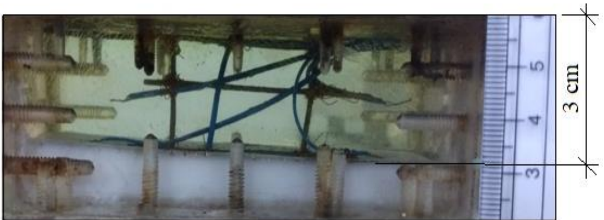
(b) Picture representing molten PCM at time t = 12 hours during heating
