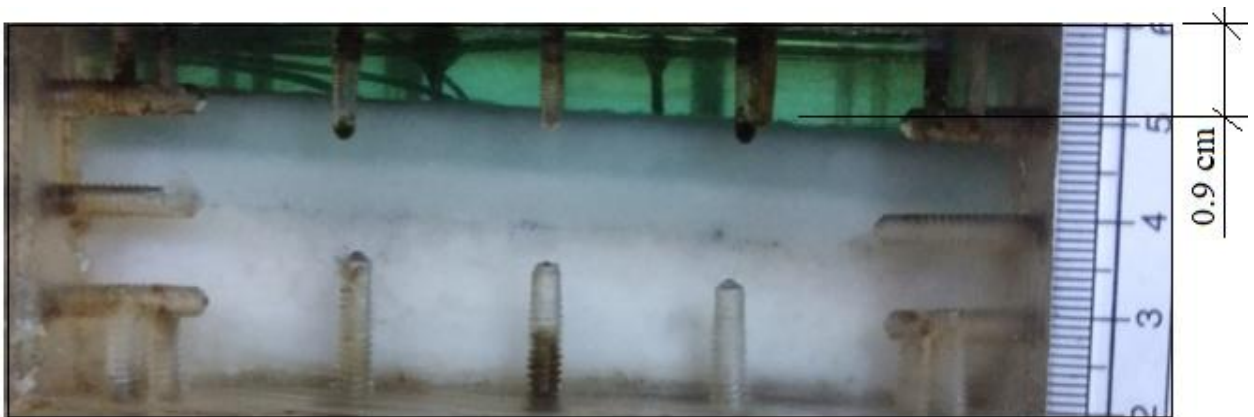
(b) Picture representing molten PCM at time t = 5:30 hours during heating
