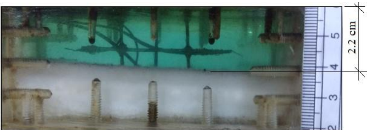
(c) Picture representing molten PCM at time t = 14:20 hours during heating
