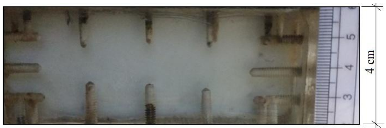
(c) Picture representing molten PCM at time t = 24:00 hours during cooling
