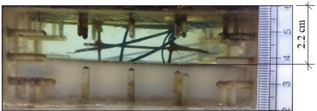
(a) Picture representing molten PCM at time t = 7 hours during heating
