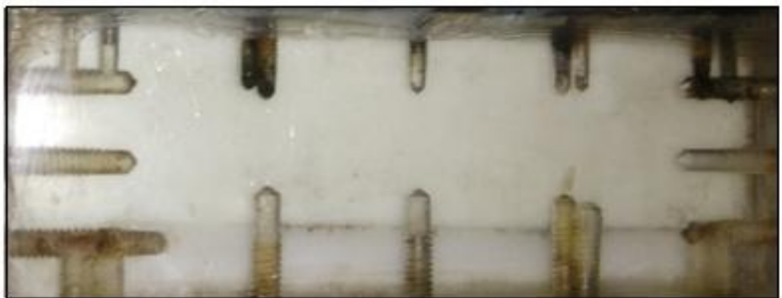
(c) Picture representing molten PCM at time t = 24 hours during cooling
