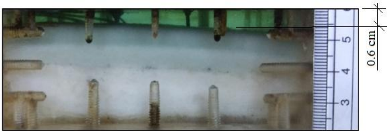
(a) Picture representing molten PCM at time t = 1:30 hours during heating
