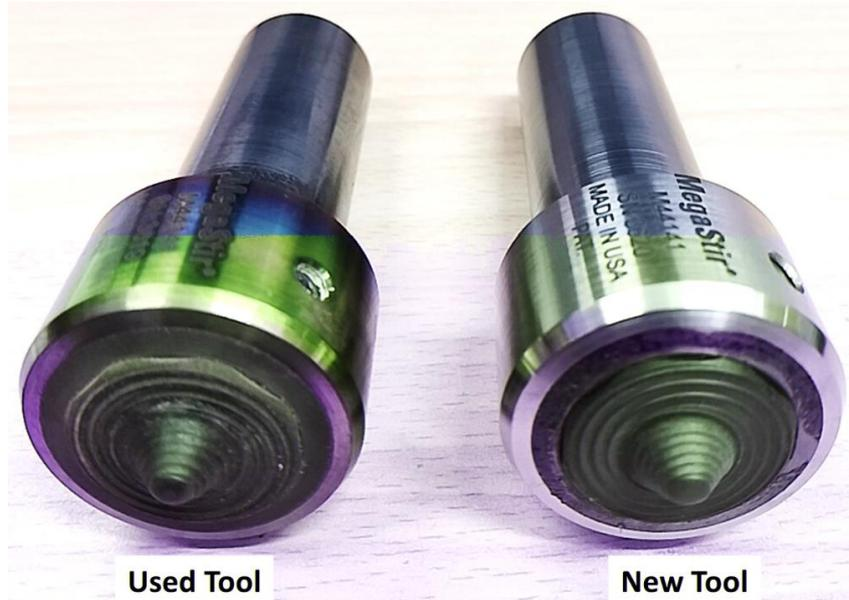
Figure 5.17 Photograph of used and new FSW tools
