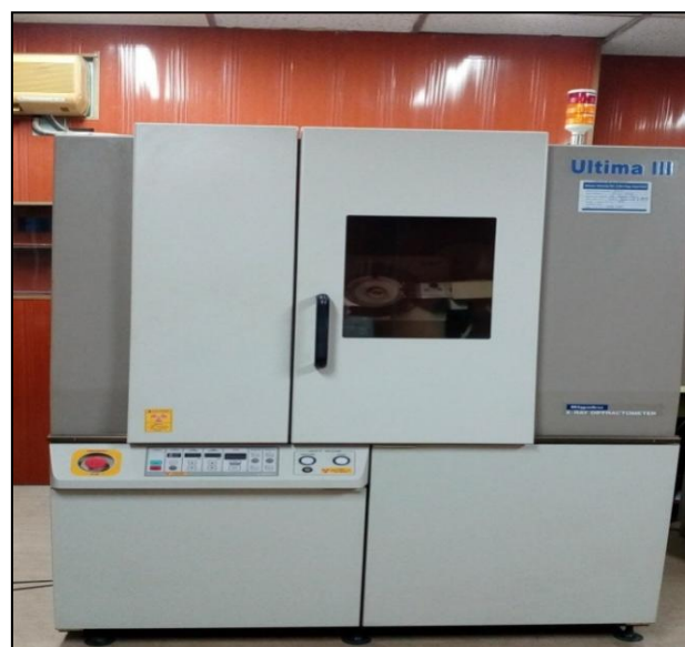
Figure 4.2 X-RAY Diffractometer [RIGAKU, ULTIMA III, 40KV, 30mA (1.2kw)] (Metallurgical and Material Engineering Department, JU)
