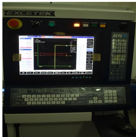
Figure 3.10 Machine control panel of EX-40 WEDM system
