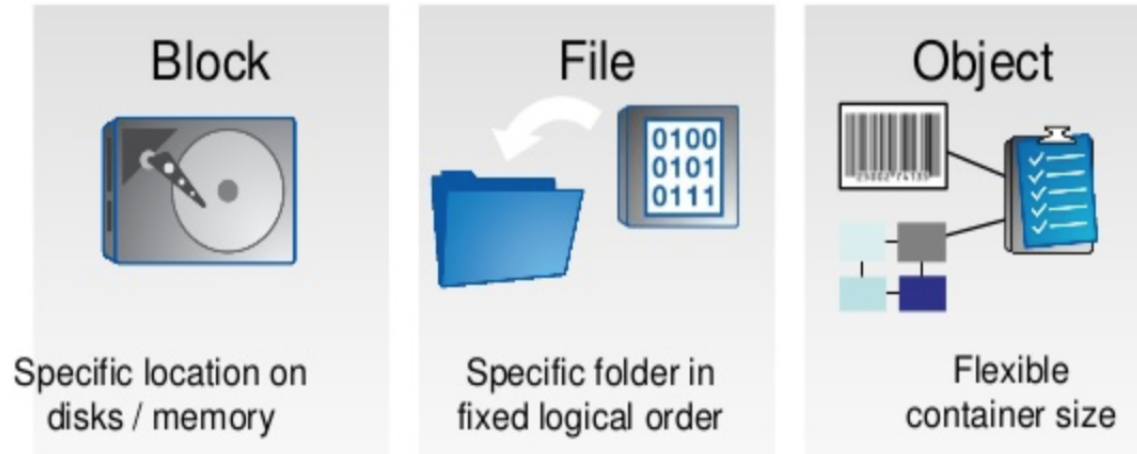
Figure 1.7: Object Based, file based, and block based cloud storage system [adopted from [39]]
