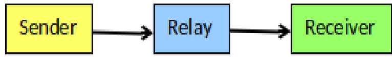
Figure 6.2: Usecase II: Sender transmits packets to the receiver via a relay node
