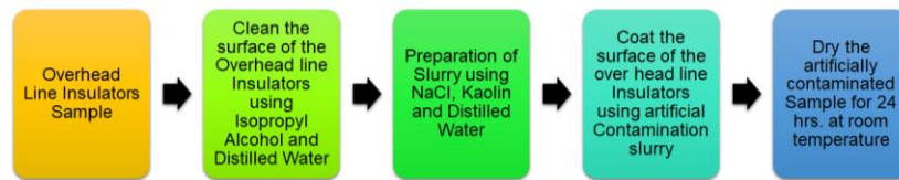
Fig. 2.3 Flowchart of artificial surface contamination process using solid layer method.
