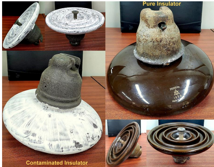
Fig. 3.1 Photography of artificially surface contaminated and uncontaminated porcelain insulators.
