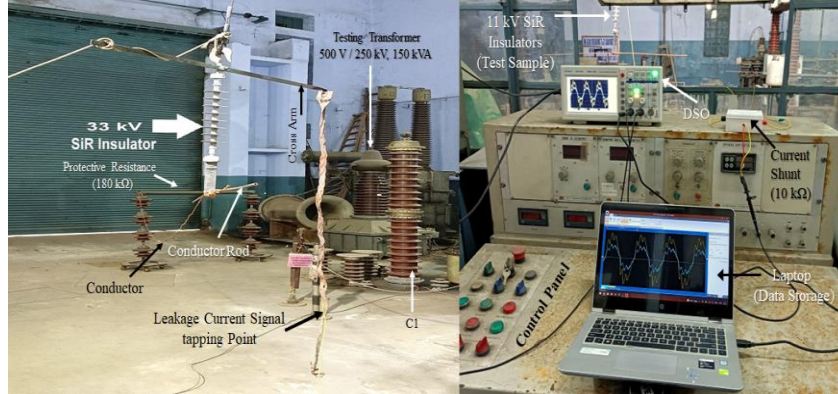
Fig. 2.4 (b) Actual Hardware setup for Surface Leakage Current (SLC) measuring system.
