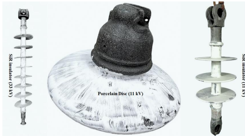
Fig. 2.2 Images of different types of contaminated overhead line insulators.
