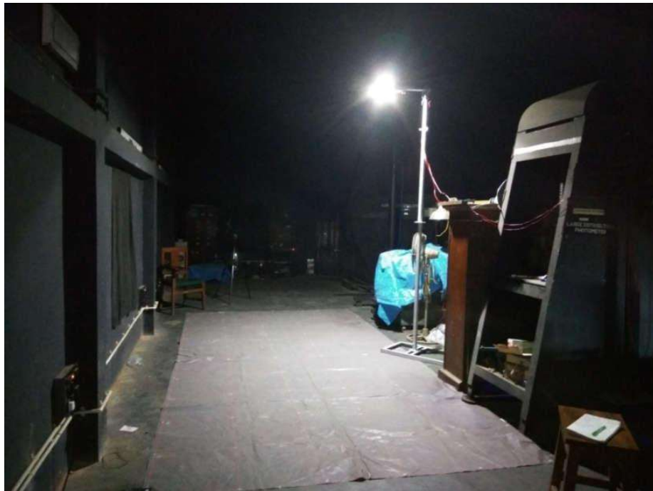
Figure 4-3. Diagram of the luminaire glowing on a flexible pole inside Illumination lab. Grid Mat has been used for measuring isolux at different PWM duty cycle
