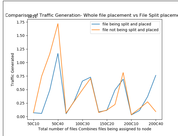
Figure 3.15: Traffic generated on a per file basis in the P2P network with no nodes in local clusters going offline
