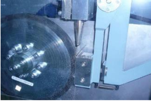
Fig 5.9: Dry Sand abrasion test and its schematic
