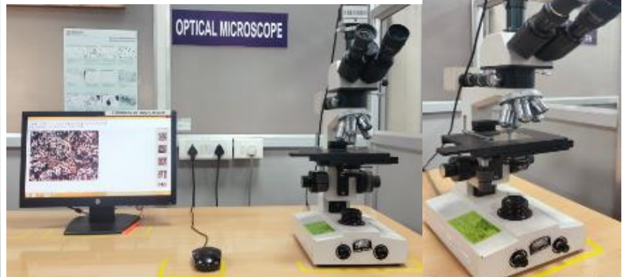
Image -03, Shows Optical Microscope with Image Analyzer Software for Microstructure analysis
