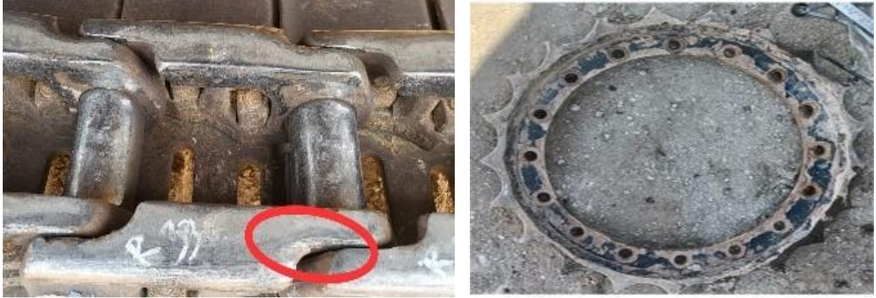
Fig 1.14 -Wear in Track link and Sprocket being ground engaging part and subjected to wear phenomenon in application
