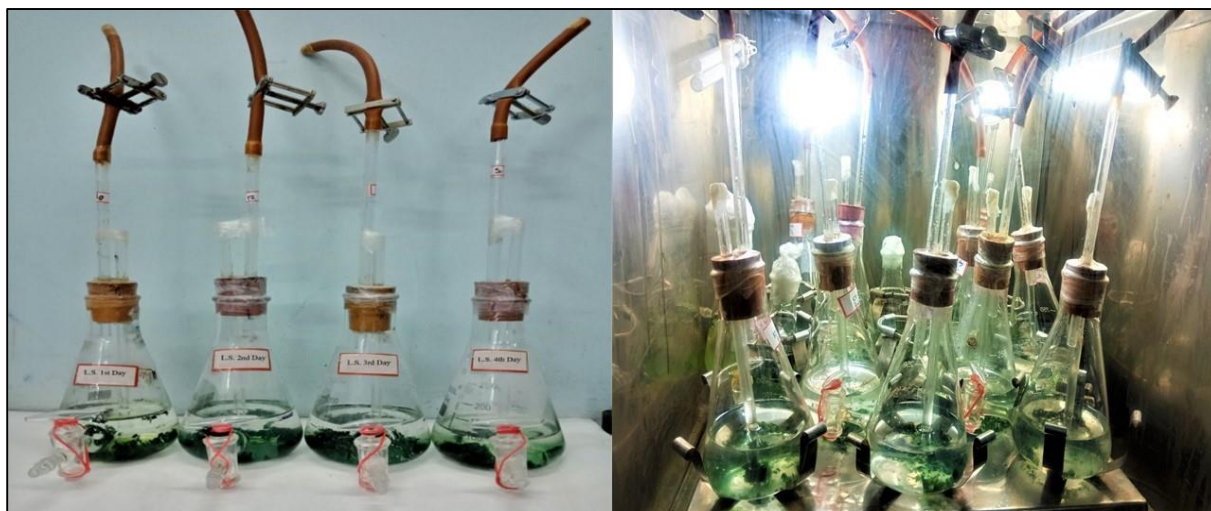
Figure 6.1. Small scale bioreactor set up for batch experiments under Photoautotrophic growth mode.
