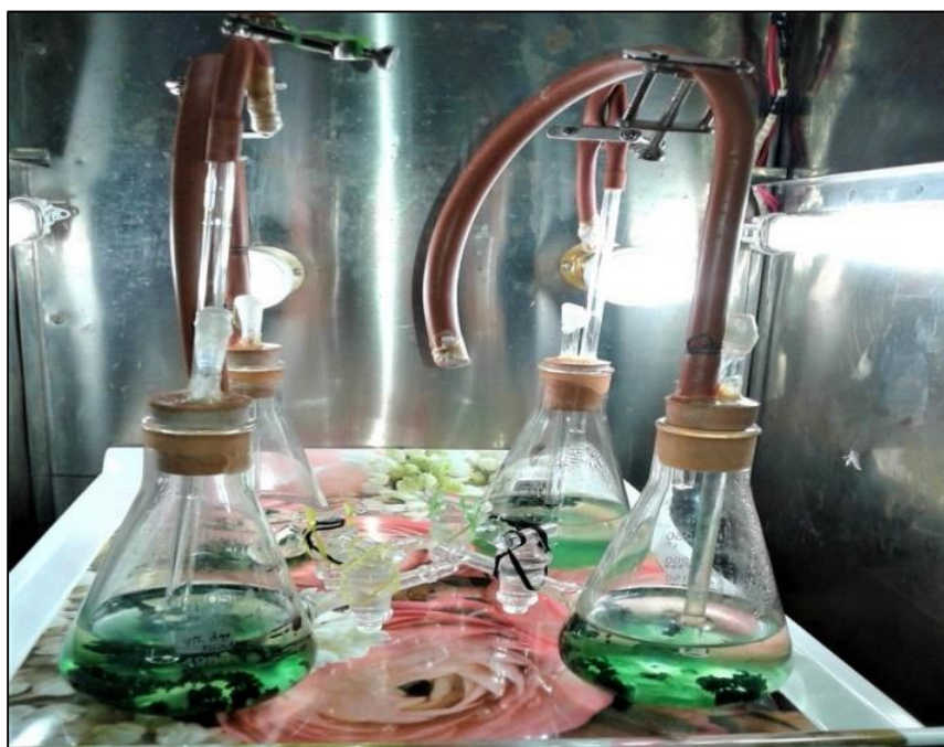
Figure 6.6 Algal growth of L.subtilis JUCHE1 at 5 th day varying different inlet-CO 2 concentrations from 5-20%v/v.
