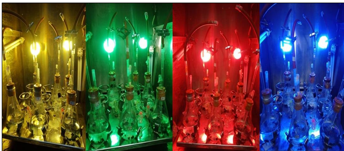
Figure 8.1. Small scale bioreactor set up for batch experiments varying different wavelengths of light.
