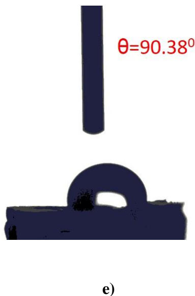
Fig. 3.4 Contact angle measurements of a) EVAM b) EVAMN5 c) EVAMN10 d) EVAMN15 before soxhlet extraction e) EVAMN15 after soxhlet extraction
