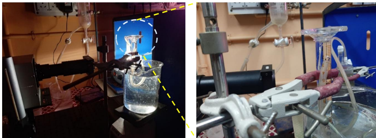
Figure 2.2: Experimental set-up for photocatalytic performance study of rGO-ZnO(1:3)/WO 3 heterojunction photocatalyst using solar simulator as visible light source
