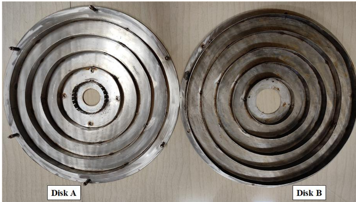
Fig 4.2: Pictorial representation of the Rotating baffled contactor (RC-1)
