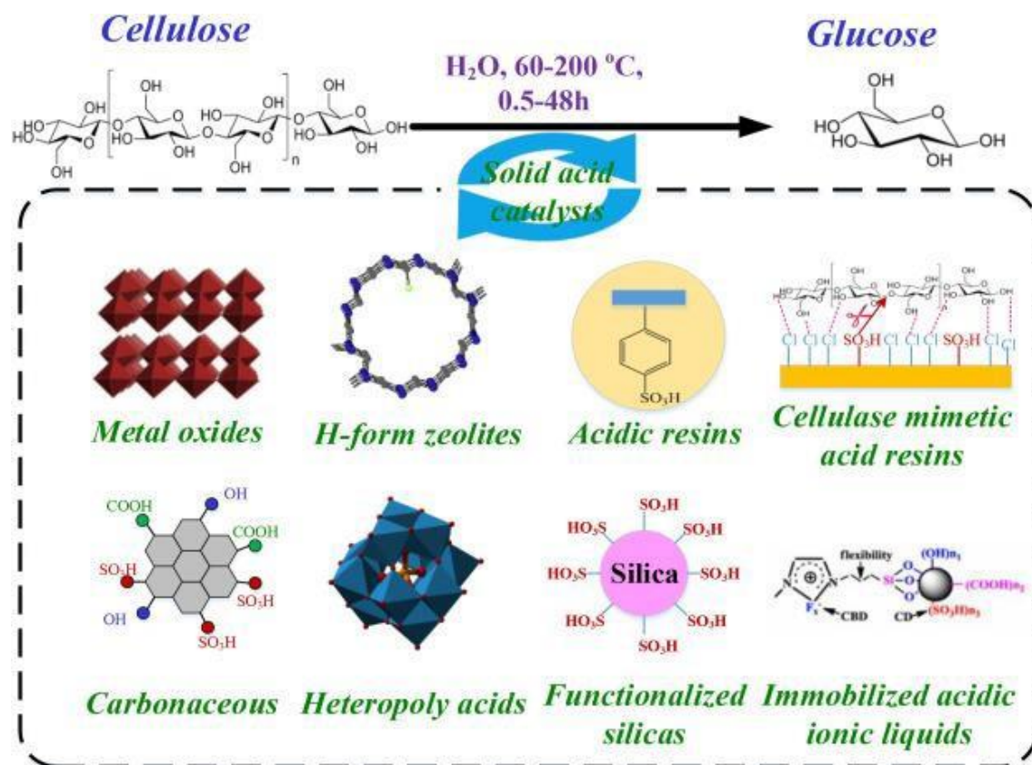
Figure 13: Solid acids used for hydrolysis (Zhou et al., 2021)
