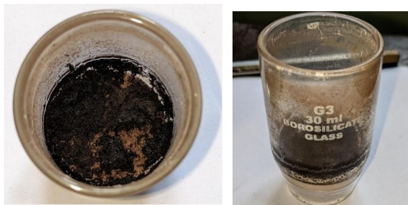
Figure 55: Extracted lignin and the Gooch crucible used to extract the lignin.
