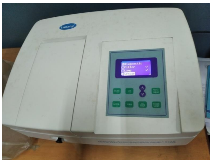
Fig.- 1.3: UV- Visible Spectrophotometer (Lassany make)
