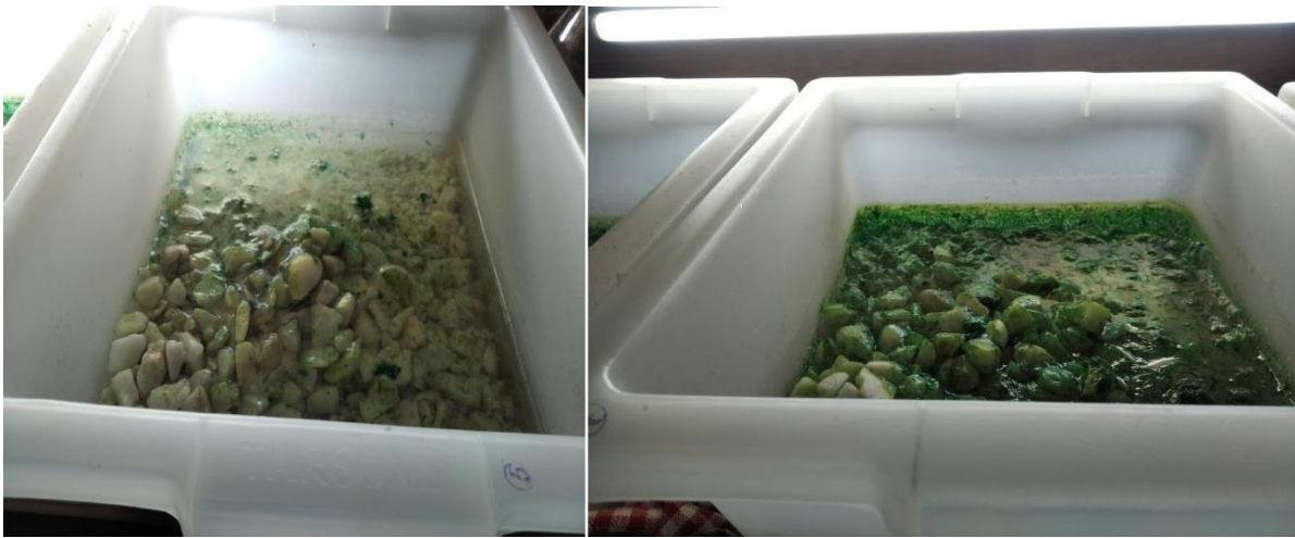
Fig. 6.2. Image of individual open air tray type Fixed film Phycoremediation Chamber
