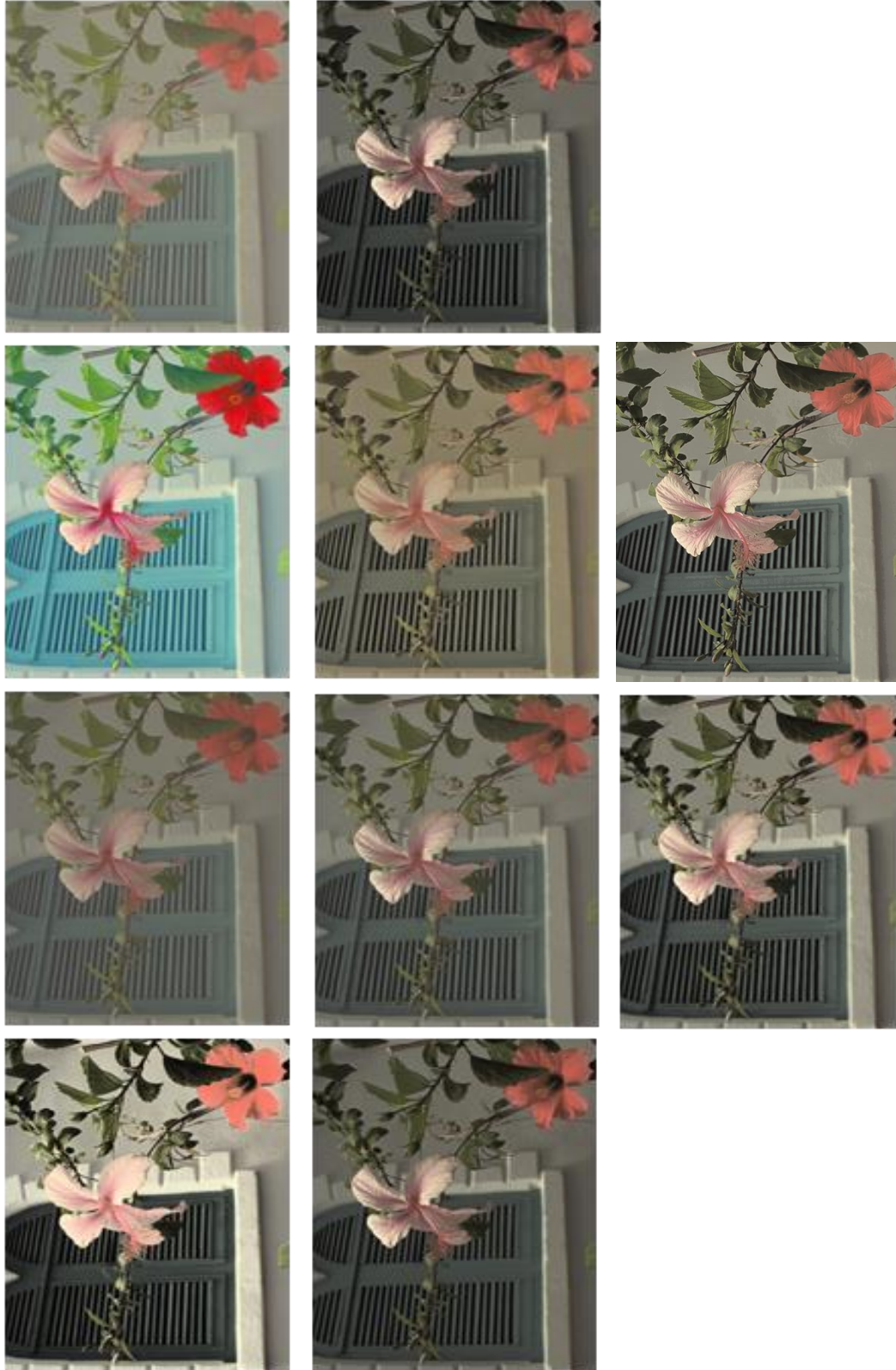
Fig. 3.8: Result of different techniques for color test image 'Flower'. (Top row from left to right) GHE, DFHE, MSR, SECEDCT, (middle row left to right) GA, ABC, CLAHE-DGCG, FDAHE-GC, (bottom row left to right) proposed BCO (using \phi ) and proposed BCO (using \varphi )
