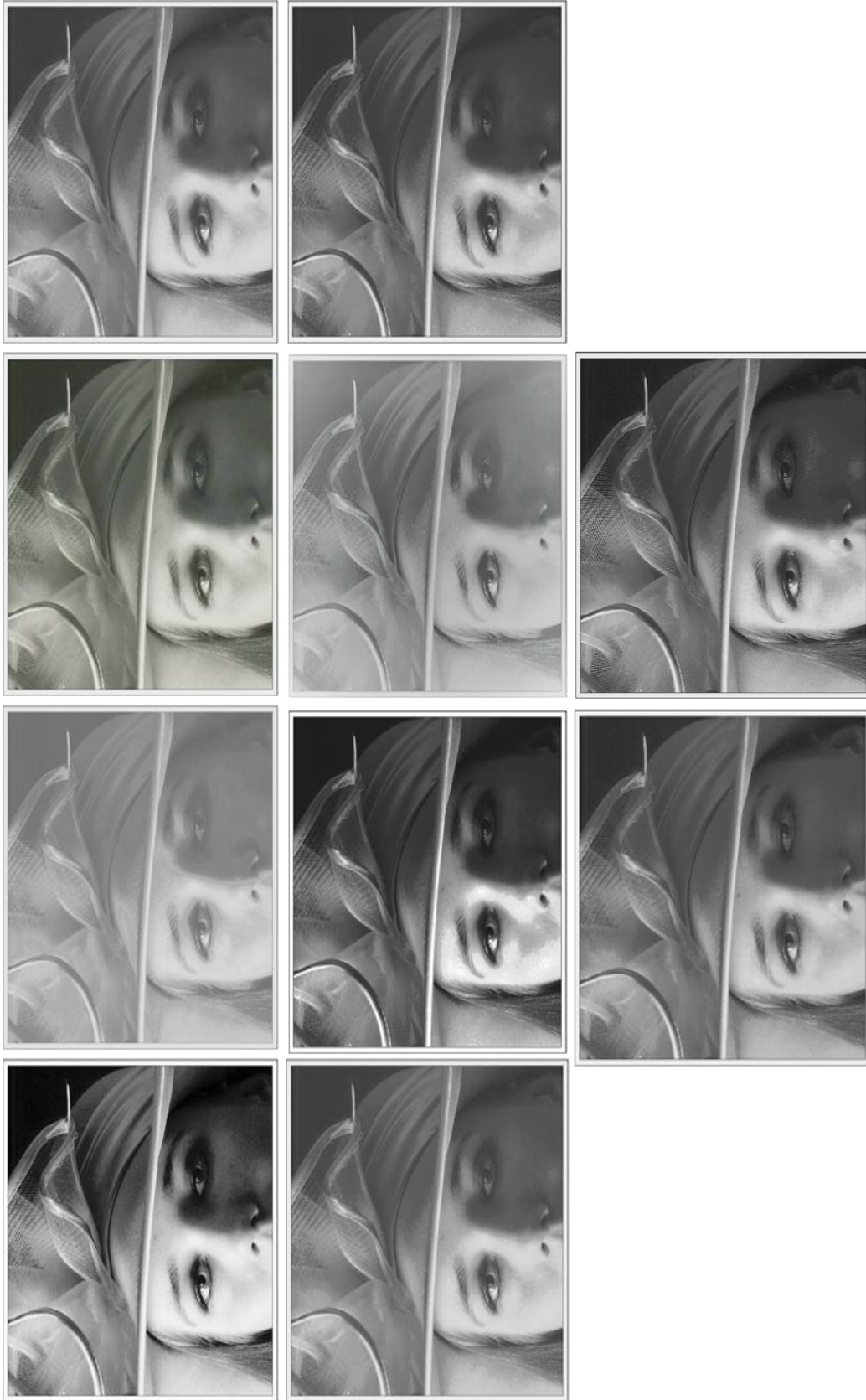
Fig. 3.7: Result of different techniques for gray test image 'Lady'. (Top row from left to right) GHE, DFHE, MSR, SECEDCT, (middle row left to right) GA, ABC, CLAHE-DGC, FDAHE-GC, (bottom row left to right) proposed BCO (using \phi ) and proposed BCO (using \varphi )
