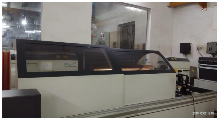
Fig 7.5: HELL machine for cylinder engraving (electromechanical)
