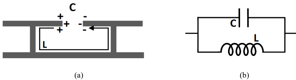
Fig. 3.2 (a) Capacitance and inductance of the unit cells and (b) equivalent lumped circuit model.
