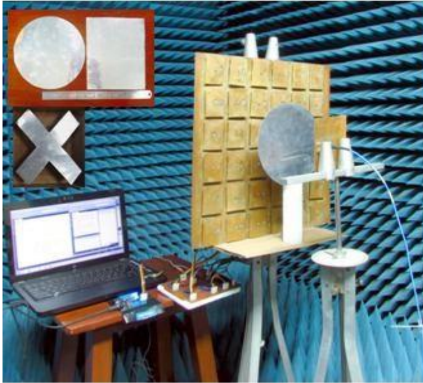
Fig. 6.17. The complete experimental setup for 2D microwave imaging system
