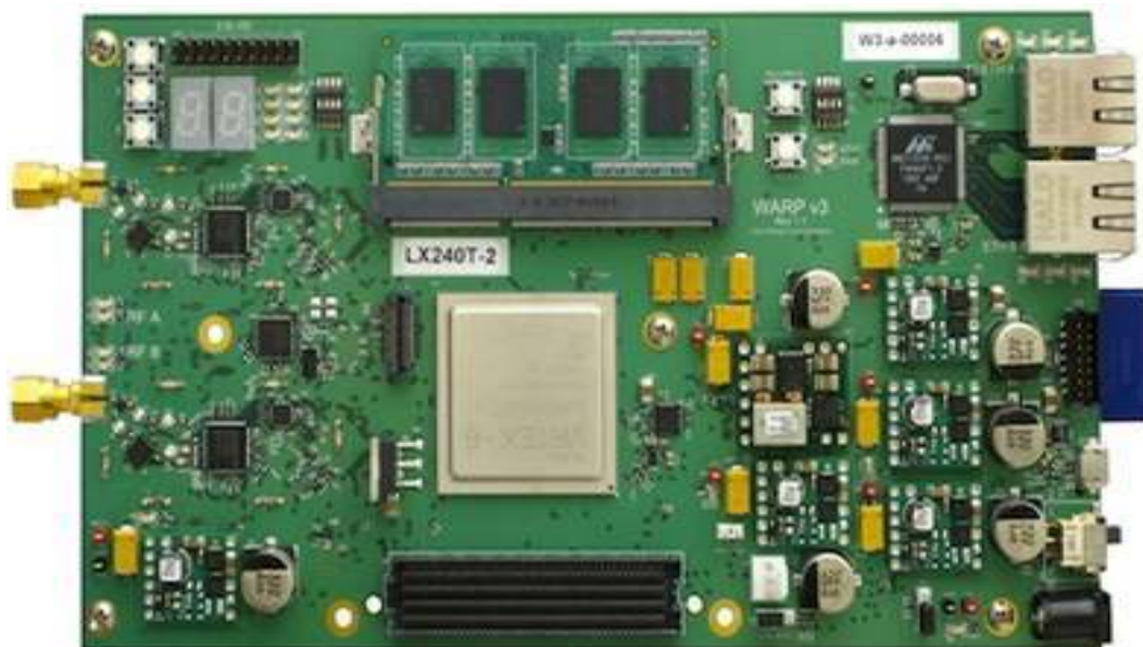
Fig. 3.3 WARP v3 SDR Board with radio daughter cards
