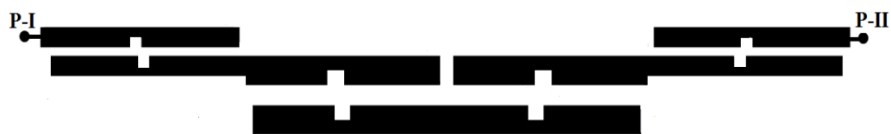
Fig. 3.69. Layout of the third-order folded PCMLBF with a single square groove.
