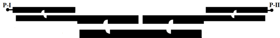
Fig. 3.113. Layout of the third-order folded PCMLBF with a single quarter-elliptical shaped groove.
