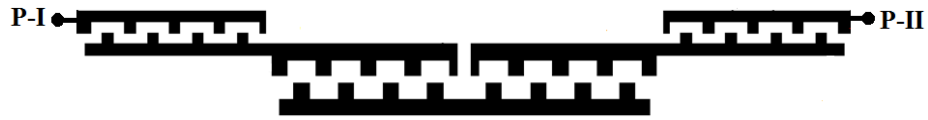
Fig. 3.137. General layout diagram for the third-order PCMLBF with periodic square shaped corrugations.
