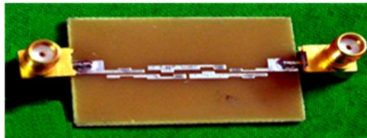
Fig. 3.214. Fabricated prototype of the third-order inline bandpass filter with asymmetric perturbation of 2-3-4-1 combination [33].
