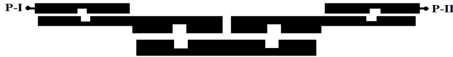
Fig. 3.83. Layout of the third-order folded PCMLBF with a single rectangular groove placed at the middle.
