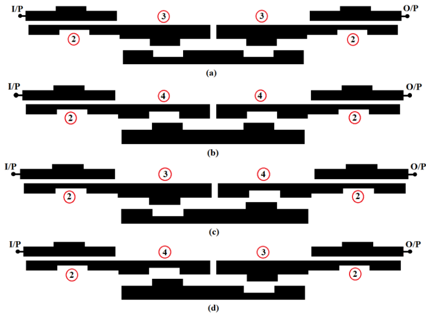
Fig. 3.190. Layouts of third-order folded bandpass filter with different combinations of asymmetric perturbations: (a) 2-3-3-2, (b) 2-4-4-2, (c) 2-3-4-2, and (d) 2-4-3-2.
