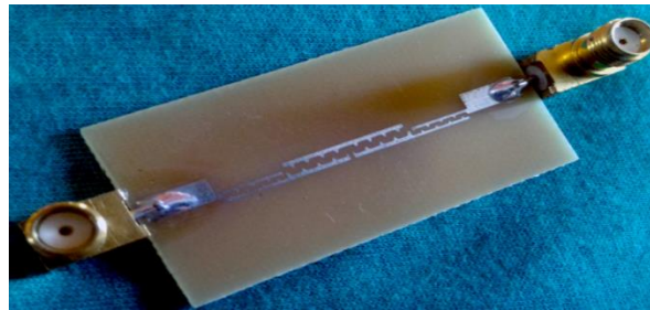
Fig. 3.175. Fabricated prototype of the third-order inline PCMLBF centered at f_0 = 5.25 GHz with four pair of periodic triangular shaped corrugations [30].
