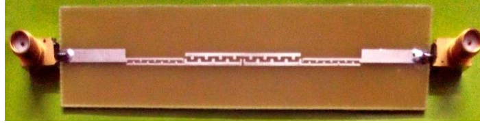
Fig. 3.156. Fabricated prototype of the third-order inline PCMLBF centered at f_0 = 2.5 GHz with four pair of periodic square shaped corrugations [29].
