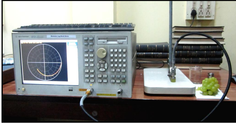
Fig. 4.12: Broadband dielectric measurement setup for grape samples at 25 °C using open ended coaxial probe technique
