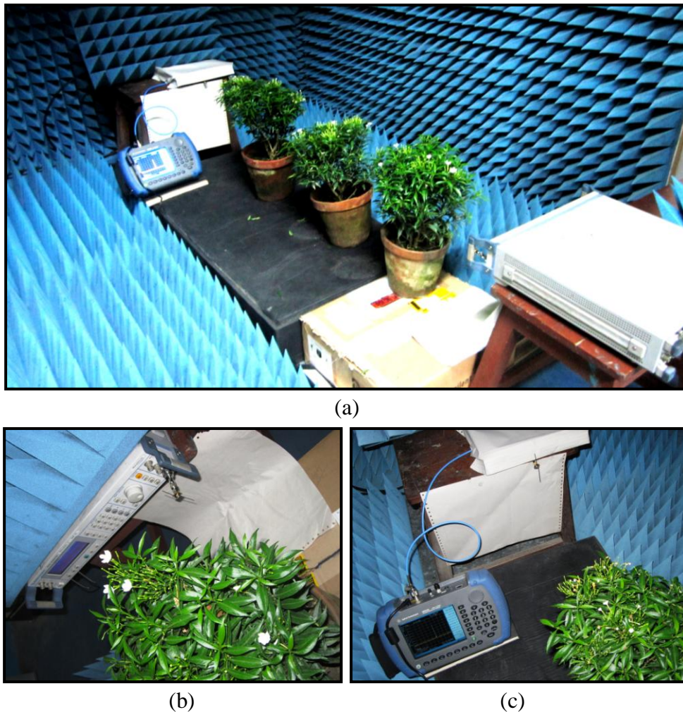
Fig. 6.3: (a) Experimental setup inside semi-anechoic chamber for measuring propagation loss due to presence of the plants, (b) Microwave signal generator with the transmitting half-wave dipole antenna at 1.75 GHz and (c) HSA connected with the receiving half-wave dipole antenna
