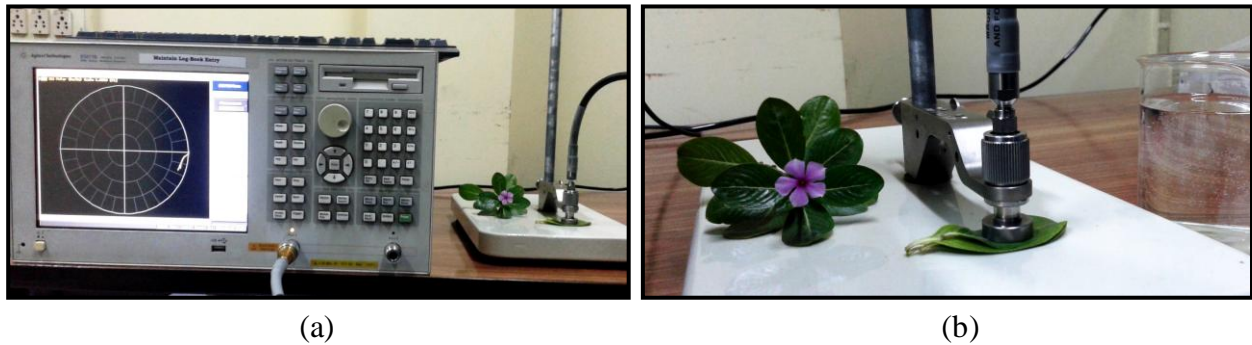
Fig. 4.20: (a) Entire dielectric properties measurement setup for Catharanthus roseus leaf samples, (b) An enlarged view of the coaxial probe with leaf samples
