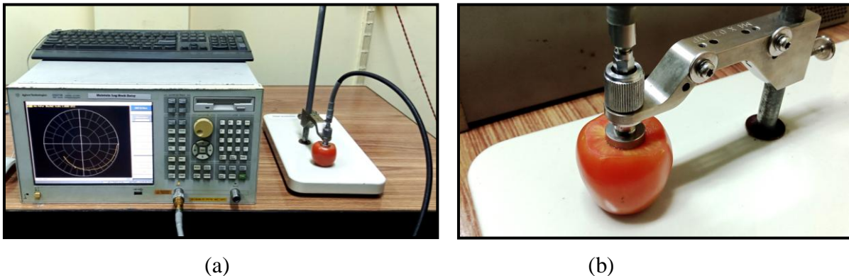
Fig. 3.18: Open ended coaxial probe setup for broadband dielectric properties measurement of ripe tomato specimen (a) total measurement setup, (b) a close-up view
