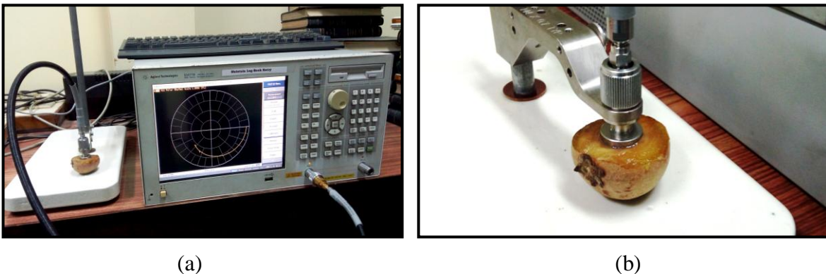
Fig. 3.12: Open ended coaxial probe setup for broadband dielectric properties measurement of sapodilla pulp specimen (a) total measurement setup, (b) close-up view
