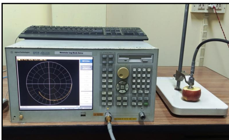
Fig. 4.7: Dielectric properties ( \epsilon_r ) measurement setup for an apple specimen
