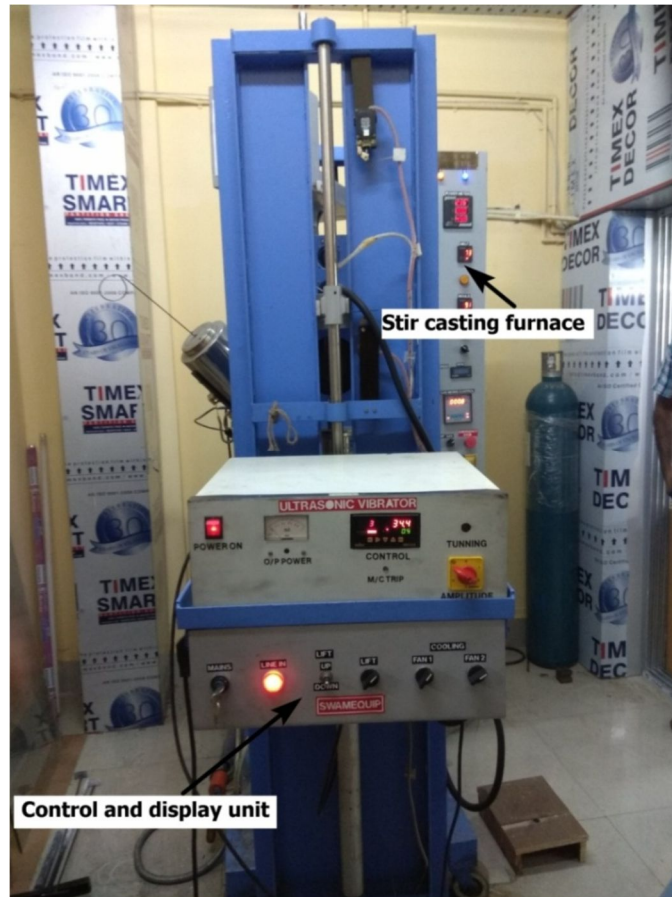
Fig 2.2 Ultrasonic vibrator to provide ultrasonic cavitation
