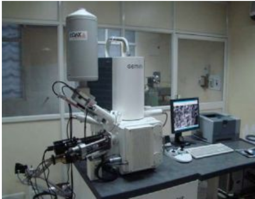
Fig 2.9 Field emission scanning electron microscope (FESEM),Supra PV35 (Carl Zeiss, Germany)
