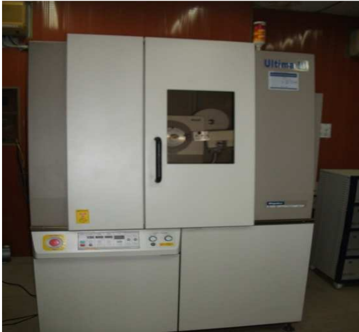
Fig.17: Rigaku Ultima III X ray diffractometer
