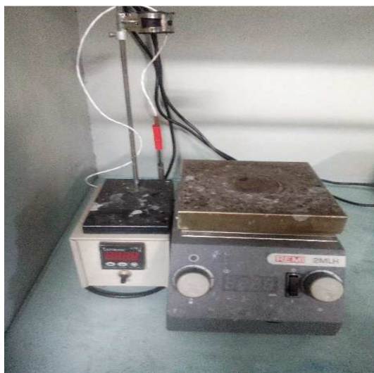
Fig.4: Magnetic Stirrer CE Model- 2MLH
