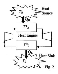
In a real heat engine, the working medium is at temperatures  $T_H^*$  and  $T_L^*$  during the heat addition and heat rejection, respectively. This is to enable heat transfers  $Q_H$  and  $Q_L$  under a finite temperature difference. If
