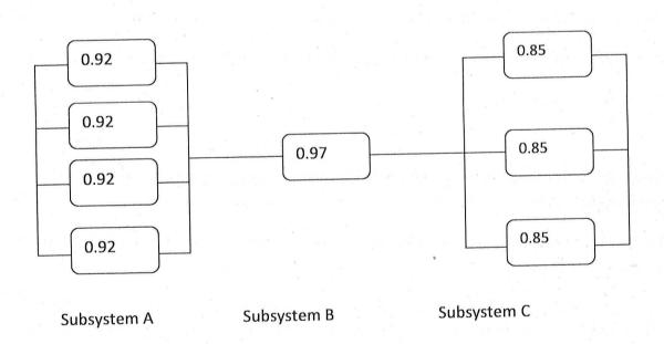
In subsystem A two components must operate for the subsystem to function successfully. Subsystem C has true parallel reliability. Calculate the reliability of each subsystem and overall system reliability.
