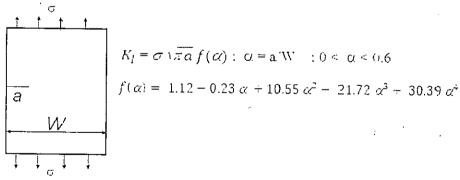
3. A 3 mm thick tension panel 10 cm wide containing an edge crack of 1 mm yielded at a load of 150 kN. However, at a load of 120kN, another panel of same material cracked into two pieces when the crack was 5 mm long. With this information, calculate the yield stress and fracture toughness of the material.
