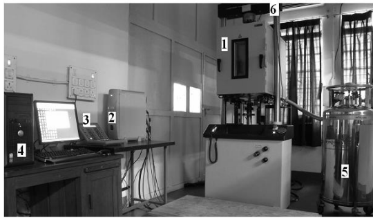
1 Cryo-chamber 2 Controller 3 Operator panel 4 Support computer 5 Liquid nitrogen cylinder 6 Temperature indicator.
