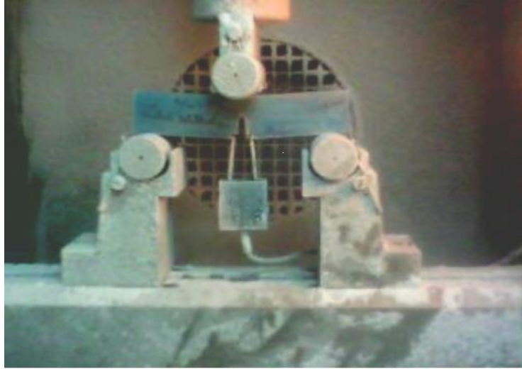
Fig.2.5 Experimental arrangement for cold temperature J_{IC} tests
