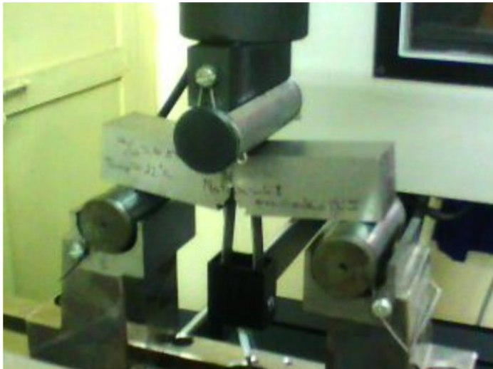
Fig 2.4 Experimental arrangement for ambient temperature J_{IC} tests
