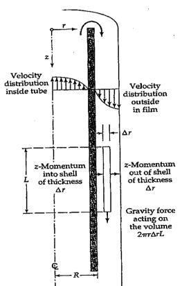
According to the associated figure, derive the velocity profile of the falling film. Find the expression of average velocity and shear stress on the wall. Find an expression for Reynolds number of the falling film. Mathematically show that between up flow and down flow streams continuity equation is satisfied,
