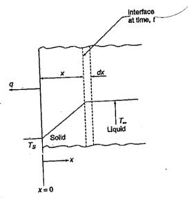
In the above figure, schematic of a solidification (moving boundary) problem is presented. In this problem liquid is being solidified. Derive a relation between the thickness of solid section as a function of time. Write proper assumptions and boundary conditions required to solve the problem.
