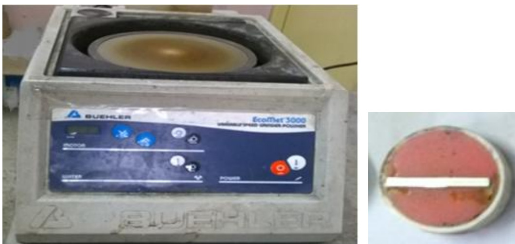
Fig. 3.5: Semi-automatic polisher and mounted sample after polish
