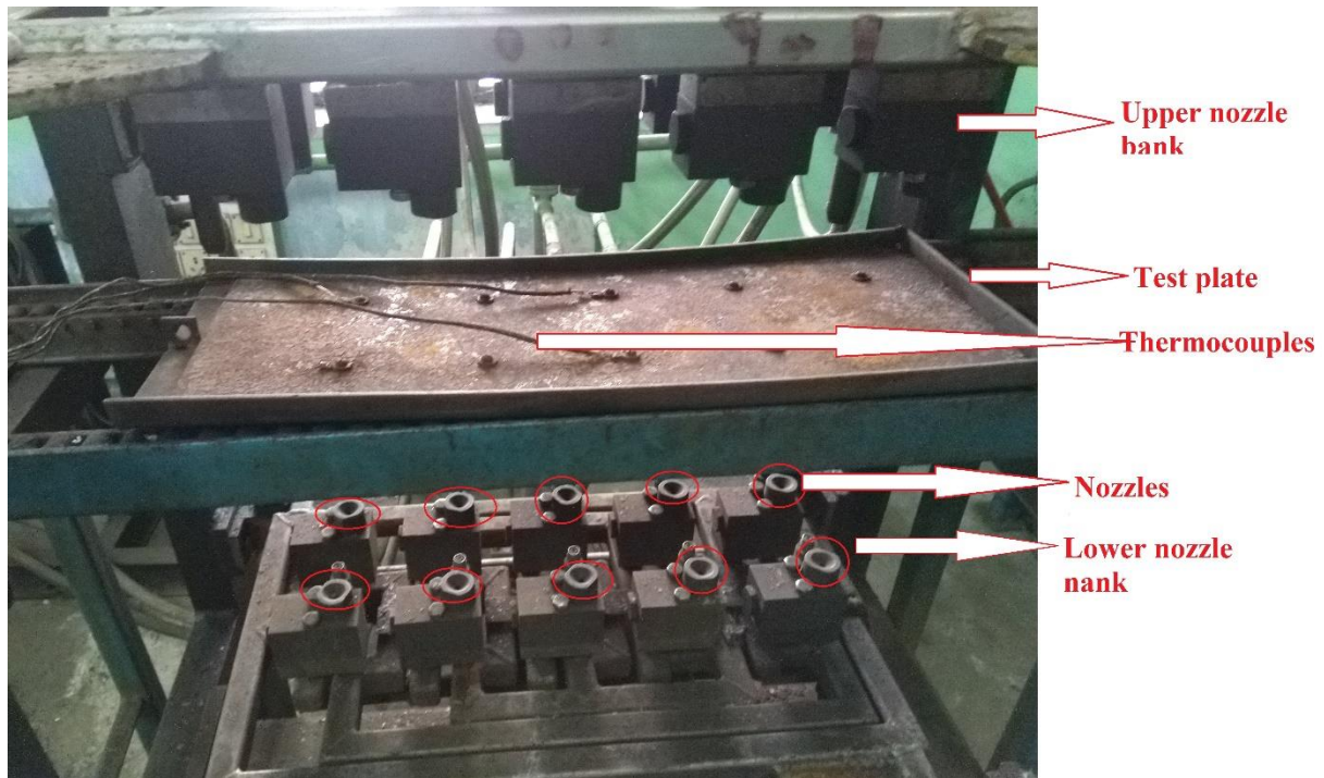
Figure 2.2 Nozzle Bank and cooling section
