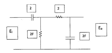
b. Using Block diagram reduction method find the transfer function [6+14 =20 marks]
