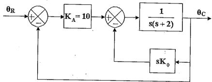
Determine the derivative feedback constant, K<sub>o</sub>, which will increase the damping ratio of the system to 0.7. What is the steady state error resulting from unit ramp input for this new setting of derivative feedback constant.
