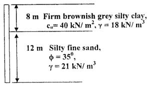
Pile is 20 m long. Take stiffness factor of pile-soil system is 5 m.
