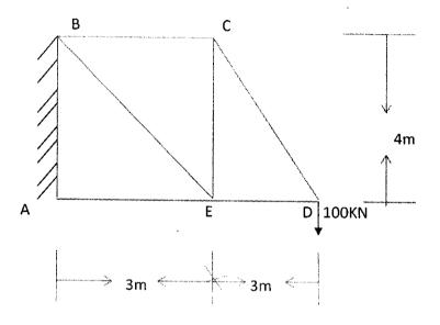
2. A) Determine the Horizontal deflection of Point A in the frame as shown in Figure. Take  $E=2X10^5N/mm^2$ .  $I=30X10^6$ .[ 15+5=20.]
