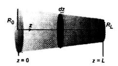
Using the lubrication approximation, determine the mass flow rate vs. pressure drop  $(w \text{ vs. } \Delta P)$  relationship for a Newtonian fluid (of constant viscosity  $\mu$ ).
