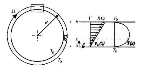
Temperature profile for viscous heat generation. The rectangular section in the flow between two coaxial cylinders can be approximated by the plane narrow slit on neglecting the curvature of the bounding surfaces.
