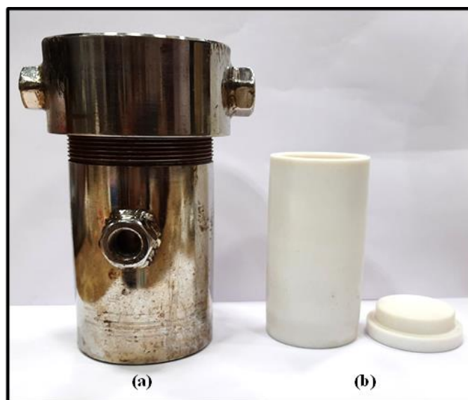
Figure 3.1: Image depicting (a) Autoclave setup and (b) the Teflon tube in the autoclave
