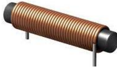
Fig. 3.3 : A standard inductance used in our measurement
