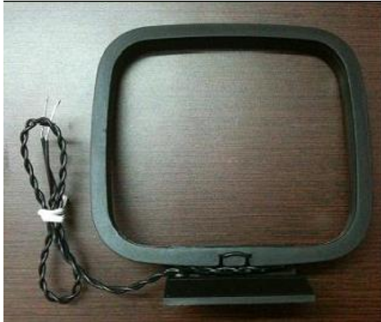
Fig. 2.2 : A standard square loop antenna
