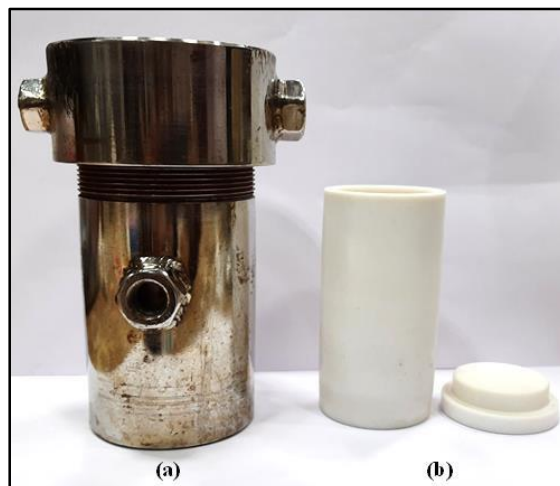
Figure 3.3 Photographs of autoclave arrangement (a) and Teflon tube inside the autoclave (b)
