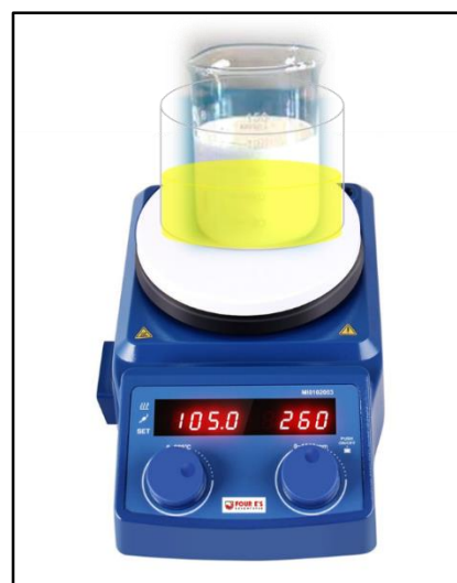
Figure 3.1 Magnetic stirrer with hot-oil bath set-up
