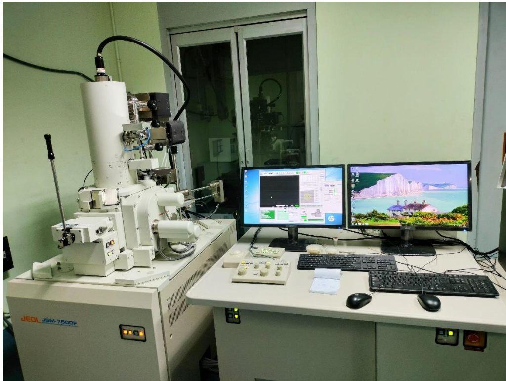
Fig. 3.8 Digital image of FESEM instrument (JEOL, model: JSM-7500F).
