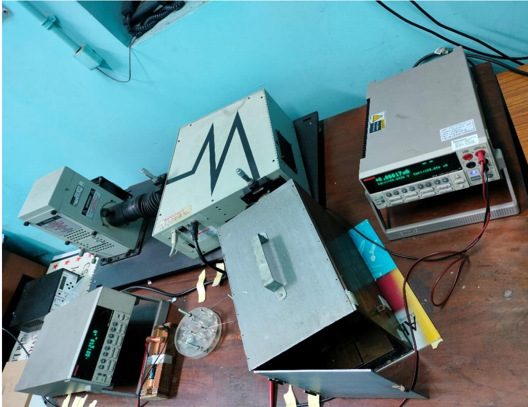
Fig. 3.24 Digital image of the photoconductivity measurement system.
