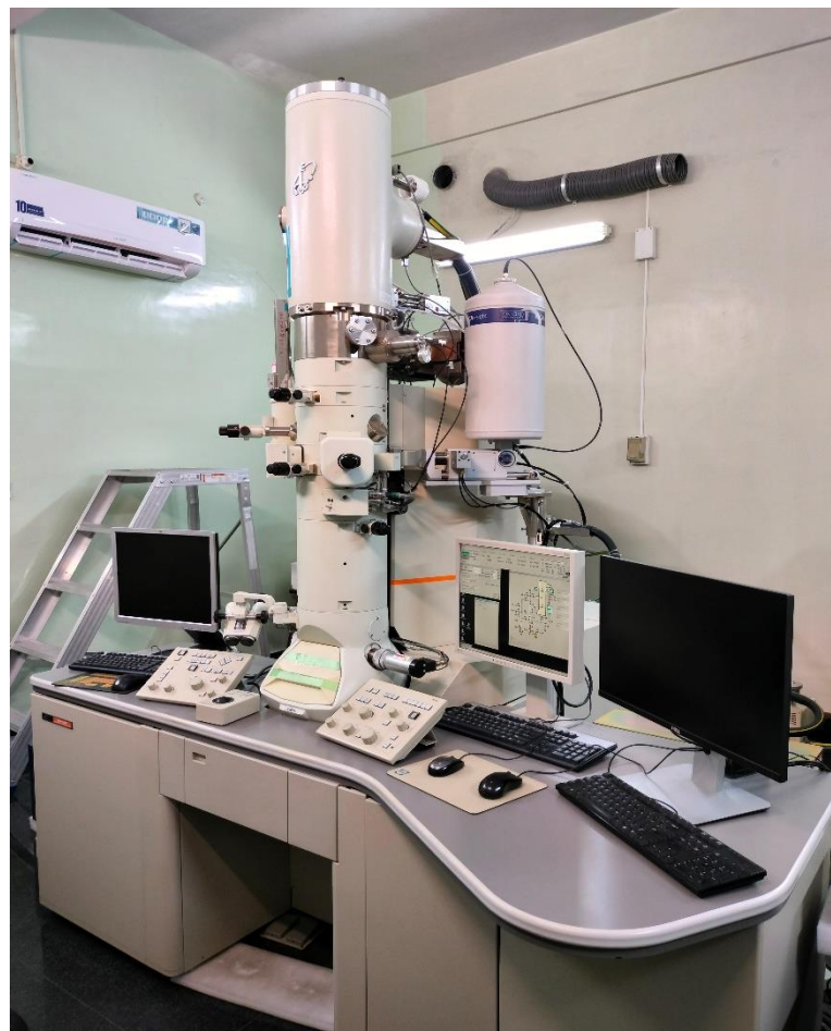
Fig. 3.10 Digital image of TEM instrument (model JEOL_JEM – 2010).
