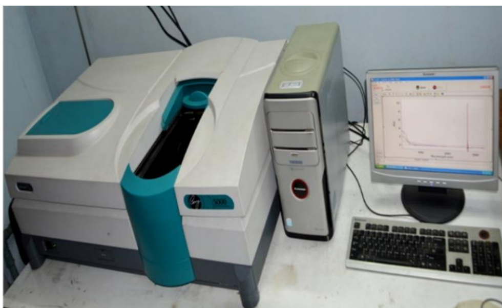
Fig. 3.16 Digital image of UV-VIS spectrophotometer (Perkin elmer, model: Lambda 35).
