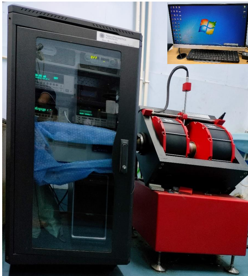
Fig. 3.22 Digital image of the Hall measurement system (Nano Magnetic Instruments).
